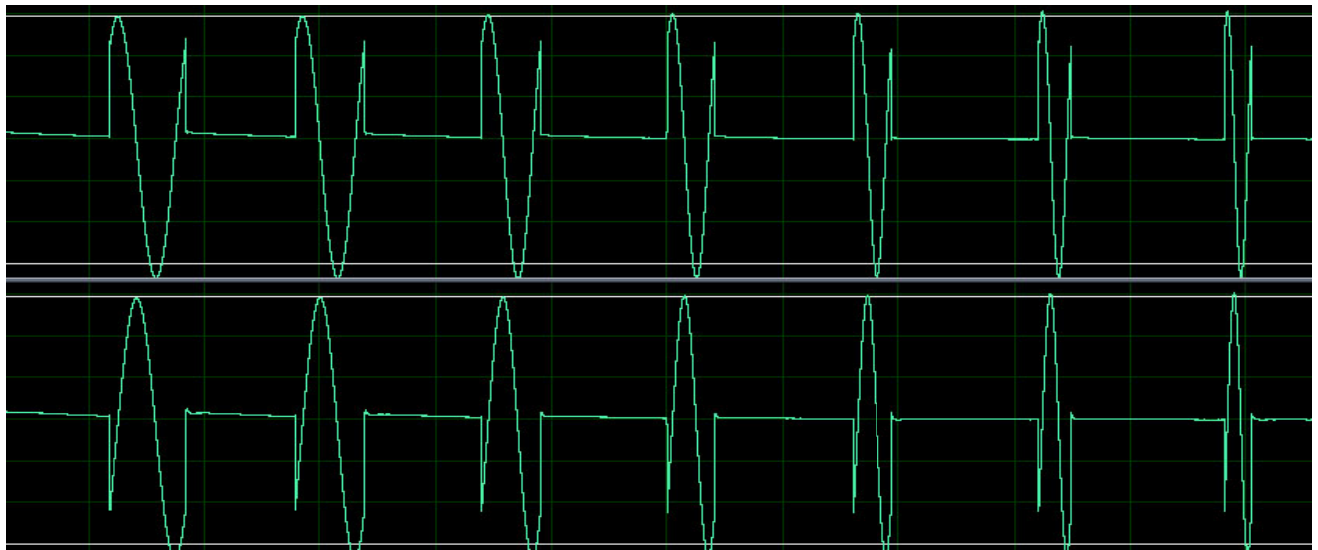
1-shot+int sync mode in output mode 0001 with OSC2 set to sinusoid. The pitch of OSC2 is increased in the right half of the figure.
