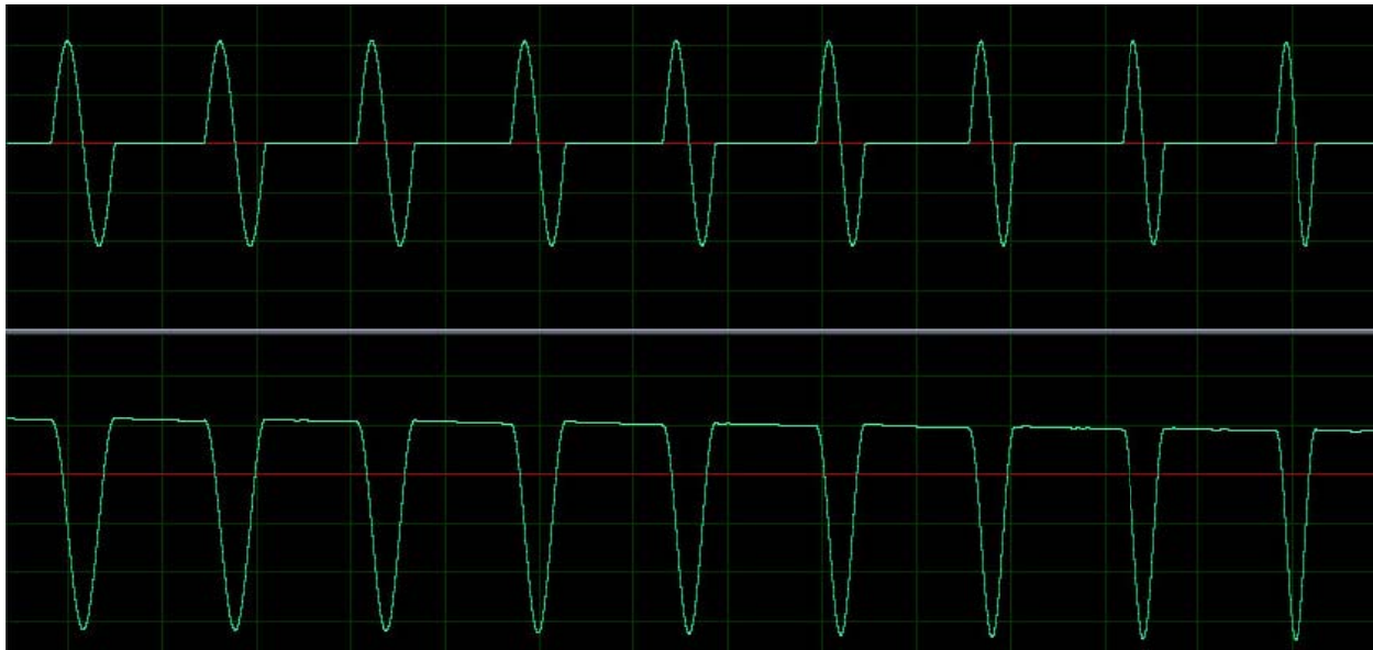
1-shot mode with OSC1 sinusoid synchronized by an external pulse train. The pitch of OSC1 is increased in the right half of the figure.
